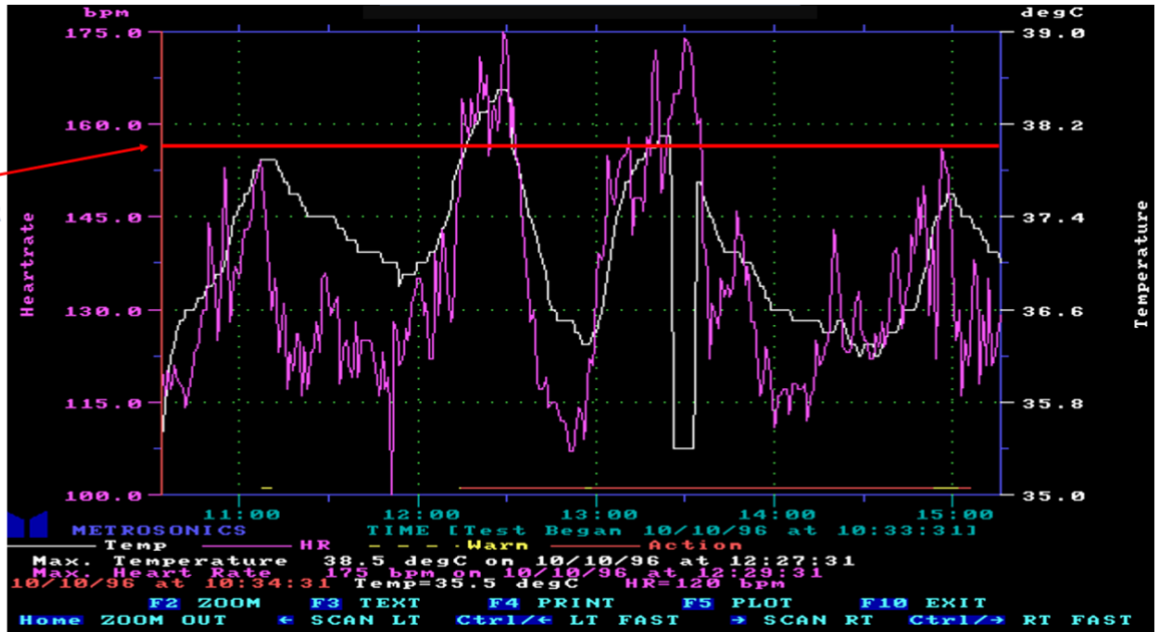
Figure A6 Physiological output from an asbestos removal. (Source: Monitor Consulting Services)
